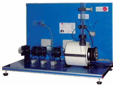
① Unit: HCCC. Centrifugal Compressor Demonstration Unit
