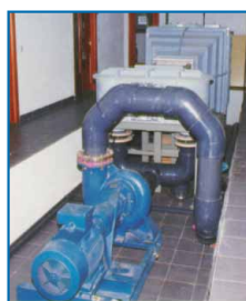
① Unit: TA500-500. Water Tunnel, 500 x 500 mm
