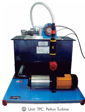
① Unit: TPC. Pelton Turbine
